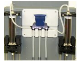
Precision syringe pumps for buffer flow
