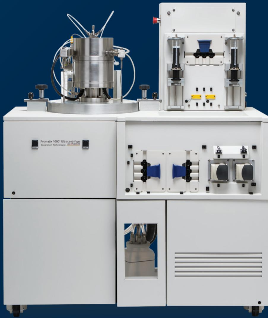
Fully programmable to run user defined applications. Fully automated for gradient and product loading, continuous flow separation, fraction collection and cleaning. The system provides operators with easy to read continuous displays of operational steps, critical run data and subsystem status.
